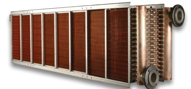
PWR Containment Cooling Coil with copper-nickel tubes, copper-nickel headers and copper fins
