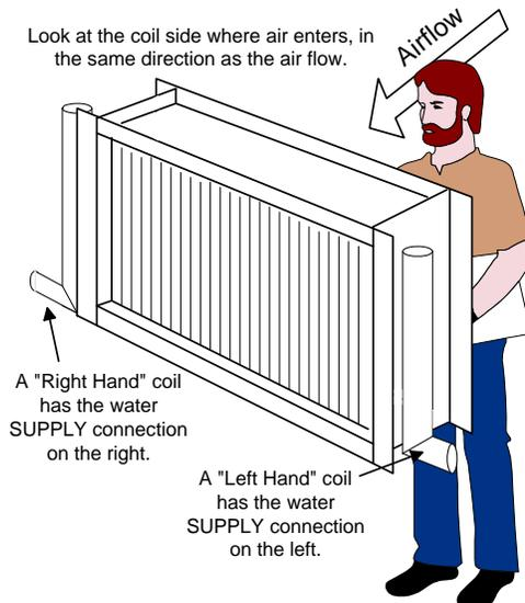
Coils can have the supply and return headers on the same end of the coil or the opposite ends of the coil. For such designs, establish the coil hand based on which end of the coil the fluid enters. Then note that the coil has the supply header and the return header at opposite ends of the coil. If not specified the coil is assumed to have both headers on the same end.
