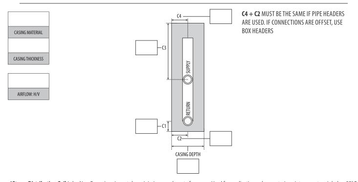
\*Steam Distributing Coil (a.k.a Non-Freeze), an inner tube; minimizes condensate freeze up. Used for applications where entering air temperature is below 32° F. Provides even air temperature on long coil lengths when steam is modulated, and /or supply and return connections must be on the same end of coil.
