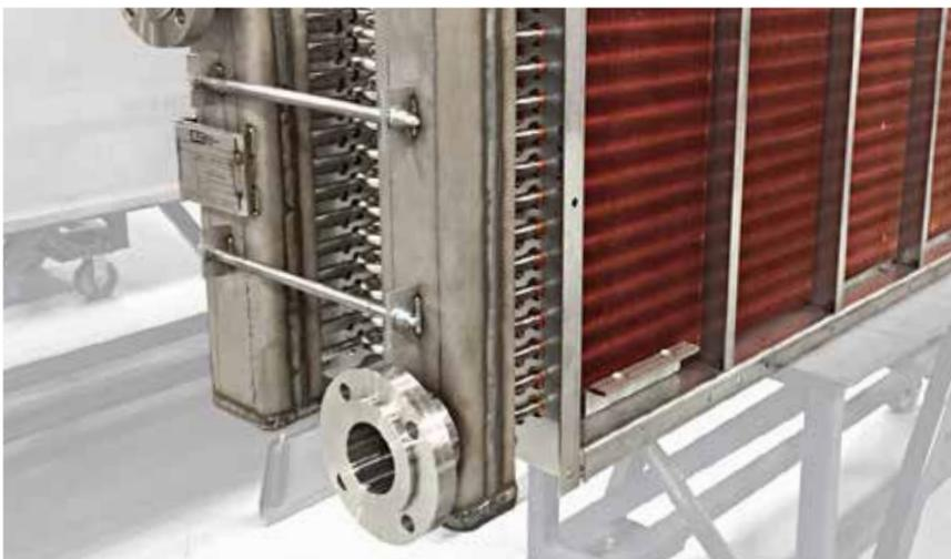
FOAK header design for high nozzle forces
