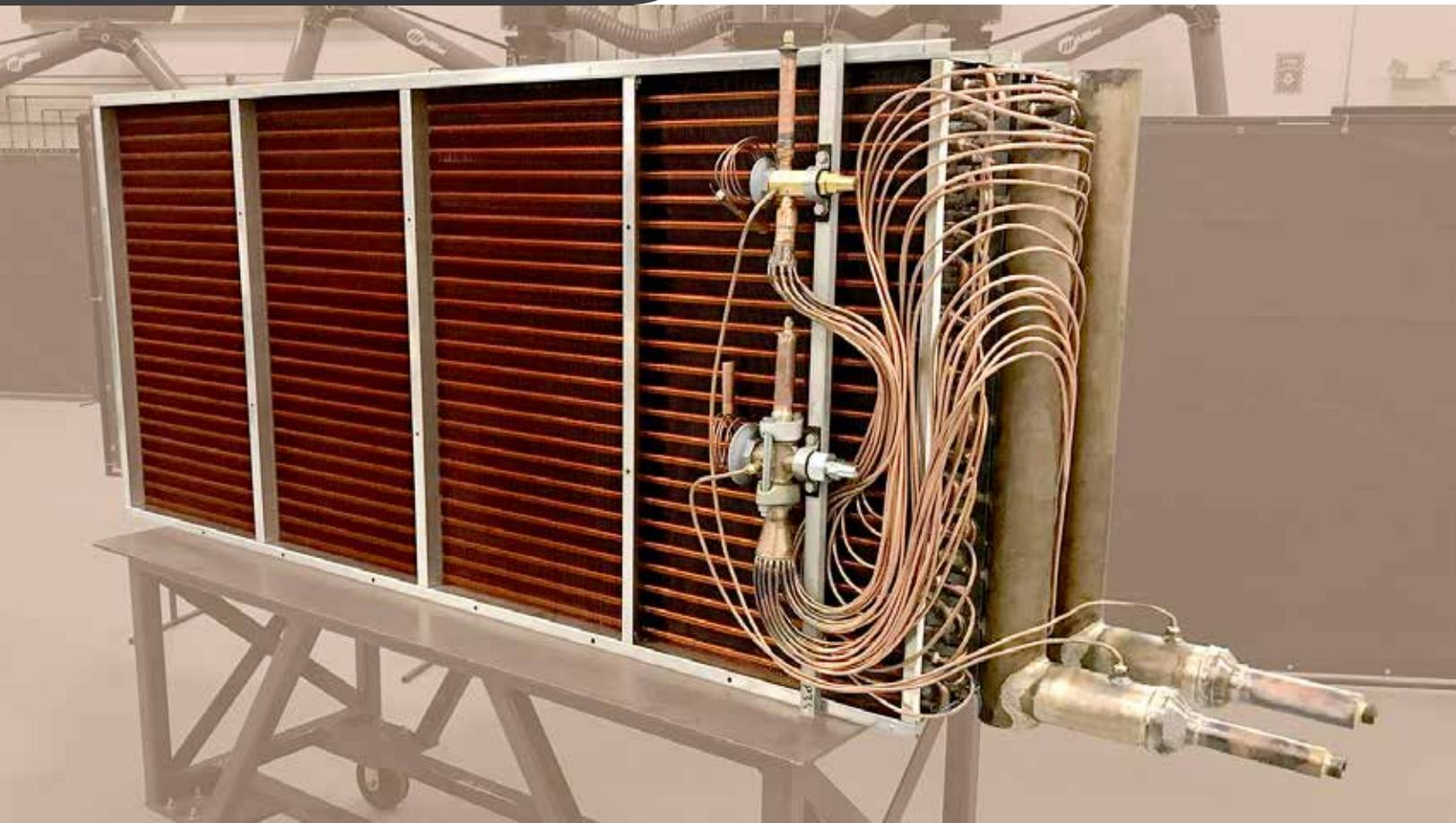
Replacement coils were needed to correct a configuration issue that reduced thermal performance in the original equipment. Restaging new coils resolved the performance shortfall while maintaining the original dimensions and interfaces.
