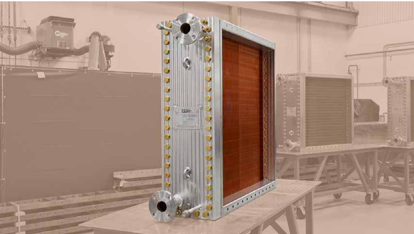
Poor-quality cooling water drove the need for new coils with ready access for internal inspection and cleaning. Removable water boxes at both ends of the coils achieved the objective. Stainless steel construction and AL6XN<sup>®</sup> tubes ensures extended service life.
