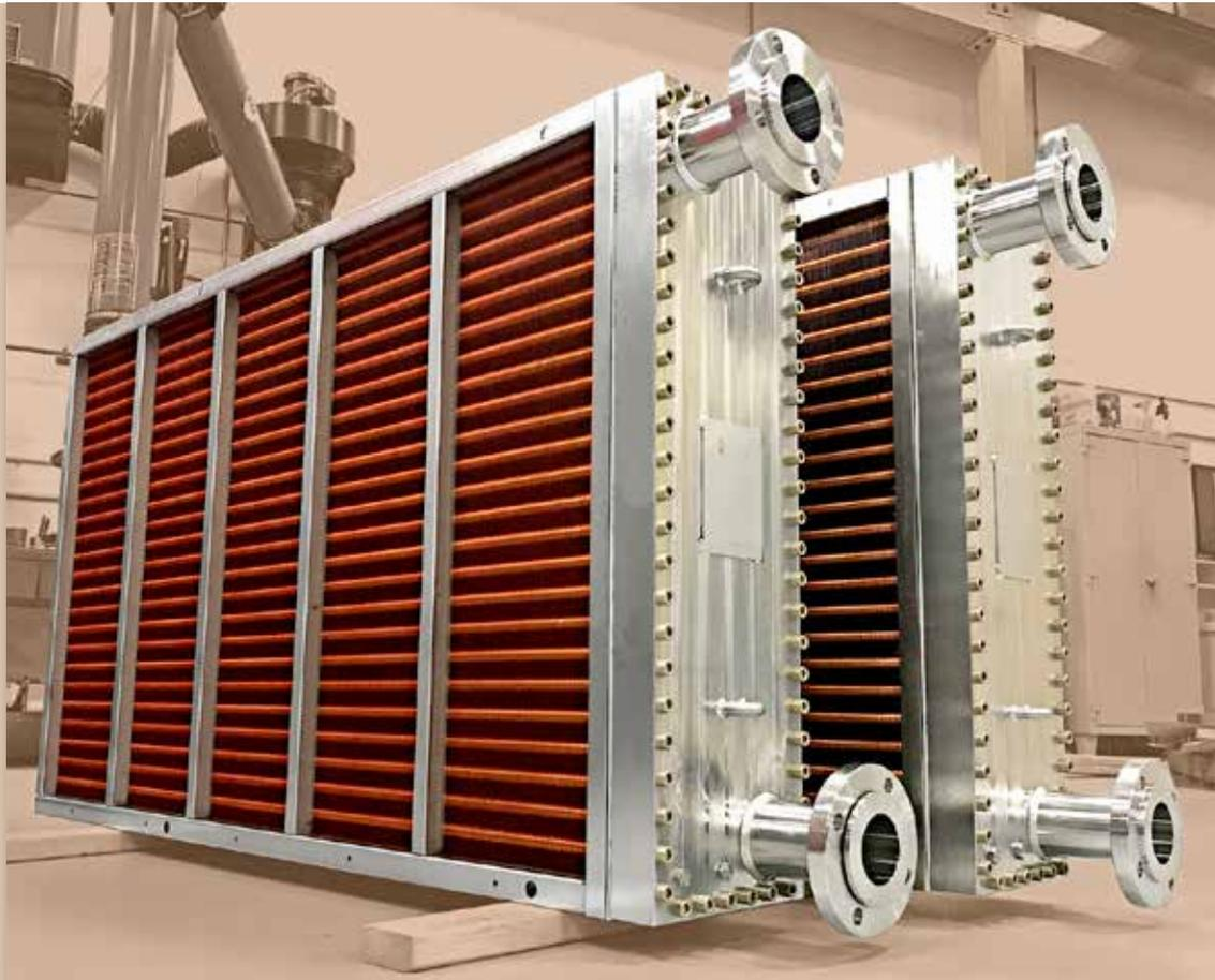
New replacement coils were upgraded with removable water boxes in lieu of closed pipe headers to address internal fouling issues.
